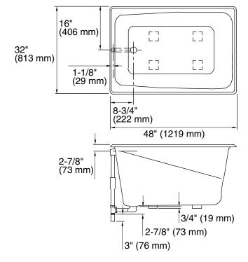
No change in measurement if connected with drain illustrated. (K-7163)
