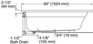
No change in measurements if connected with drain illustrated. (K-7272)
