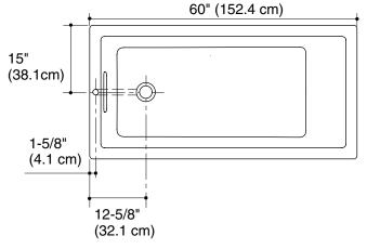
No change in measurement if connected with drain illustrated. (K-7272)
